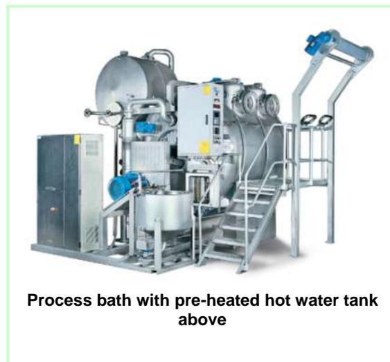
Use the lowest practical temperatures to reduce the time taken for heating, and drain machines at the highest practical temperatures to reduce the time for cooling and use of cooling water. It is important to buy machines with appropriately sized heat exchangers. If they are too big, heating and cooling can be too fast and if they are too small heating and cooling can be too slow.
