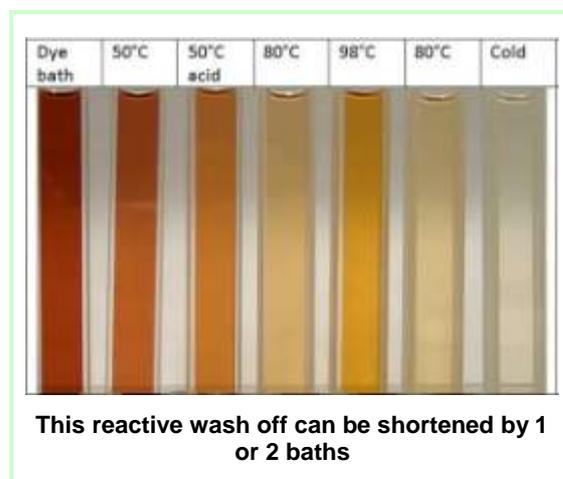
The best rinsing option is combined cooling and rinsing. In this method small amounts of fresh water are introduced into the dye vessel and then a small amount of water is released down the drain. This discontinuous process gives the fresh water time to mix with the dye liquor so the washing effect is efficient, and the introduction of cold water is a quick way to cool machines resulting in a water and energy efficient process.
