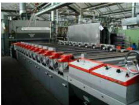
Rotary screen printing with integral dryer
